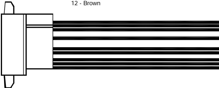
You should make all electrical connections to the wiring harness before installing the connector on the amplifier. If the amplifier ever needs service, the connector can be easily removed from the amp without unwiring it.
