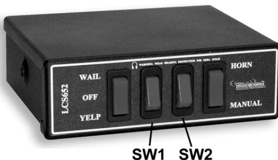
**Please Note:** *The two red wires on pins 4 & 8 (LCS652 only) supply the power for the devices switched by SW1 and SW2. Connect the red wires from Pins 4 & 8 through an appropriate user supplied fuse (up to 20 amps). It is **highly recommended** that you appropriately fuse these input wires. Damage to the siren caused by shorts in the devices connected to SW1 or SW2 will not be covered under warranty.*
