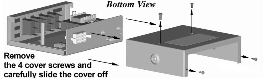
Once the cover is removed, you may move the necessary jumpers over from the “Extra” slots.
