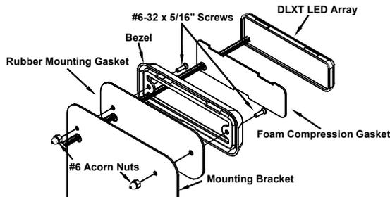
3. Mount the DLXT light(s) on the bracket as shown above. Use the two #6-32 x 5/16" screws through the back of the mounting bracket as shown. Secure the screws using the two #6 acorn nuts. Repeat for additional lights, if applicable.
