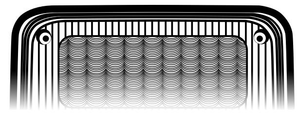
\*Light should be oriented with overlapping circles facing downward to direct light toward ground
