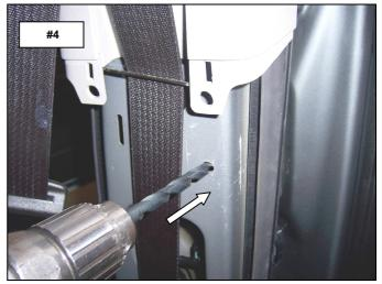
**STEP-4** INSERT (1) T-BOLT THROUGH THE RETANGULAR OPENING IN THE B-PILLAR AND POSITION IT SO THE BOLT EXTENDS OUT THROUGH THE DRILLED HOLE. ATTACH THE BRACKET TO THE B-PILLAR USING THE T-BOLT (1) 3/8" FLAT WASHER, (1) 3/8" LOCK WASHER AND (1) 3/8" HEX NUT. PHOTO'S #5 & #6
