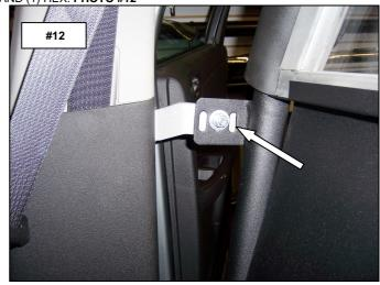
STEP-9 TIGHTEN THE PARTITION BRACKET AND SEAT TRACK NUTS AND BOLTS.
