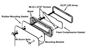
3. Mount the DLXT light(s) on the bracket as shown above. Use the two #6-32 x 5/16" screws through the back of the mounting bracket as shown. Secure the screws using the two #6 acorn nuts. Repeat for additional lights, if applicable.
